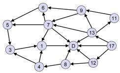
Note that positive labels can be chosen such that higher labels point to lower labels (and the destination label D = 0).
